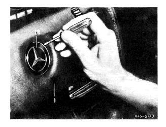
2 Unscrew hex. nut (3) and remove spring washer as well as steering wheel from steering shaft (2).
