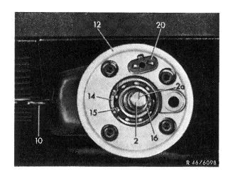
5 Place hex. nut in a socket wrench, mount spring washer and glue to socket wrench with adhesive tape.
