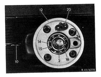
5 Place spring plate on steering shaft, screw-on hex. nut and tighten to specified torque.
