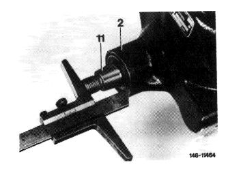
4 Screw guide sleeve (050) on drive shaft.
