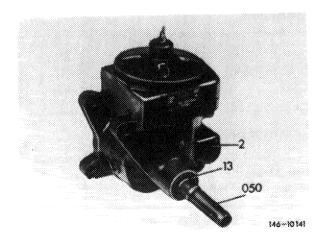
5 Screw back hex. screw of puller (050) and slip device on drive shaft, while punching with claws (051) through sealing lips of radial sealing ring (13).
