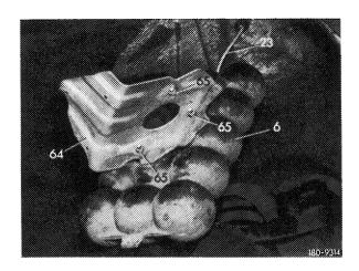
8 Screw vacuum supply tank (6) with bracket (64) to wheel house sheet metal by means of hex. nuts (63).
