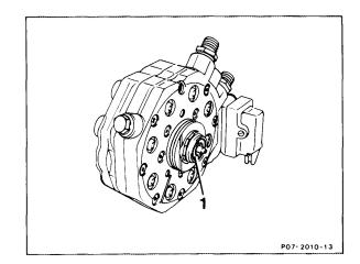
Position (arrow) of screw plug ..... measure with depth gauge and note. Mark position with scriber to be sure.
