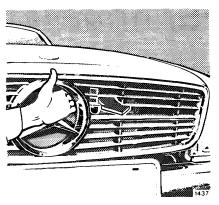
Reach through the opening of the star in the grill and pull the safety catch lever behind the radiator grill in the direction of the arrow, and raise the hood (be sure that wipers are resting on windshield).
